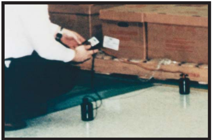
6. Resistance measurements taken with a megohmmeter confirm that the electrical properties were unchanged.
